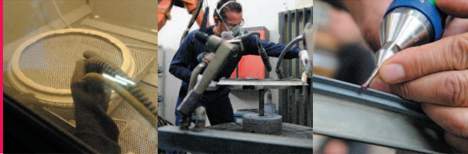
CRMA, an AFI KLM E&M Center of excellence for engines part and module repairs, has developed an innovative solution under which worn-or-damaged Low Pressure Turbine (LPT) Rotating Air Seals on CFM56 series engines are repaired instead of being replaced. Called Repair 004, it involves weld build-up of seal teeth using an automatic gas tungsten arc welding procedure.
